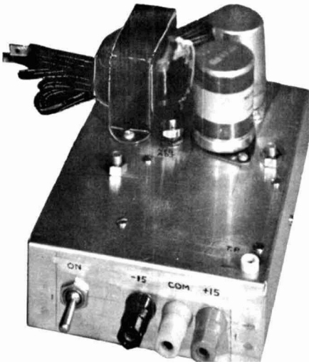
A dual IC-regulated power supply which provides plus and minus fifteen volts.
