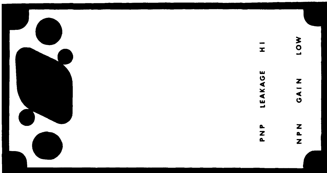
fig. 3. Full-scale photo master of the front panel for use with 3M Scotchcal. If you don't have access to photo-engraving, normal construction may be used with rub-on letters.
