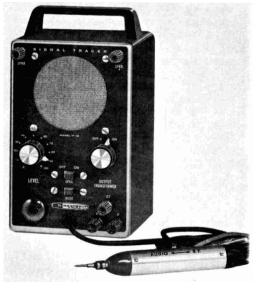
Kit-model signal tracer is high-gain (and quiet) audio amplifier. Probe can be used direct or with switch set for demodulation.
