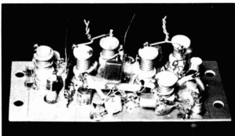
The 144-MHz FET converter; noise figure below 2.5 dB.
