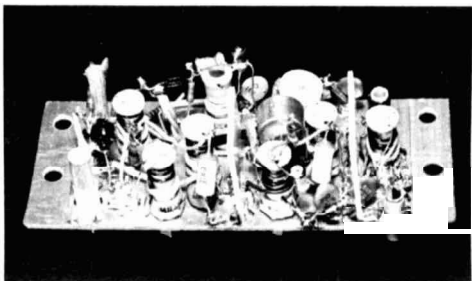
Layout of the 220-MHz converter. Input coil and neutralizing coil to the right; oscillator at top center.
