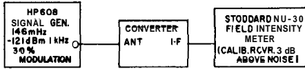
fig. 3 Test setup used to measure the sensitivity of the two-meter converter. Noise figure of the unit was calculated to be 1.52 dB.
