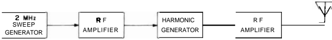
fig. 10. Block diagram of an effective defeater/jammer . A 2-MHz sweep generator circuit sweeps 1 MHz each side of center. This is amplified to drive a harmonic generator, thereby sweeping through the spectrum from 1 MHz to beyond 400 MHz. Result is complete blanketing over so wide a frequency range that few bugs escape obliteration.
